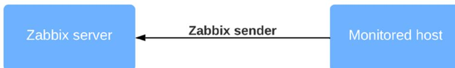
Figure 3.28 – Zabbix server trap receiver diagram
